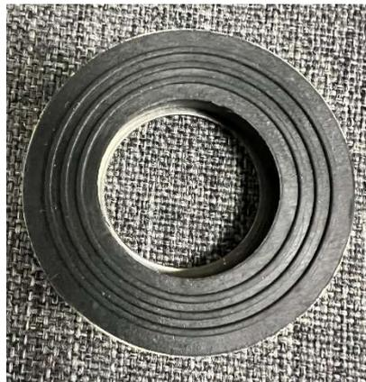
Put the part with the metal upwards back onto the thread of the faucet (rubber seal facing down towards the plate), place the other sealing part on the yellow nut and then screw it onto the thread.
