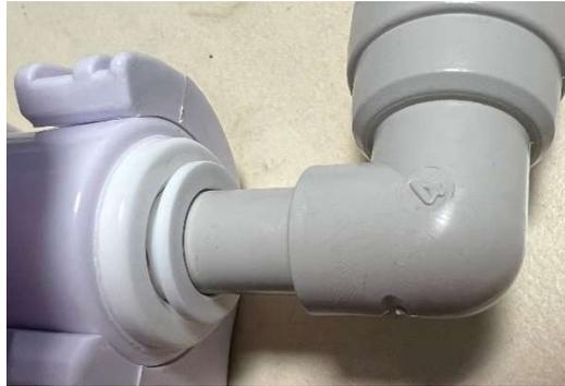
Pull slightly on the hose or elbow to create a gap in the lock.
