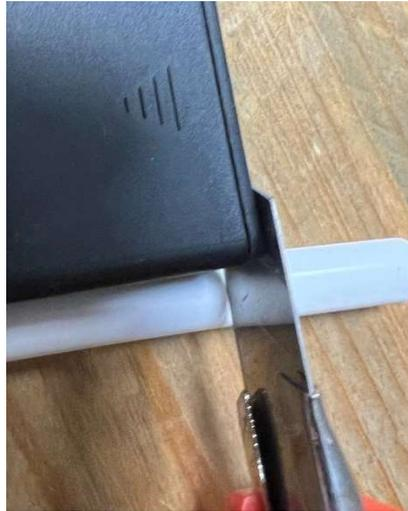
The interface of the hose should be clean and not frayed. In addition, it should be rectangular. Take a piece of thicker, straight wood or plastic and place it on the board. Position the hose as shown in the photo and cut downwards at a 90° angle. The sharper the knife, the better the result! **Please do not use pliers or side cutters! This causes the hose to deform at the interface.**
